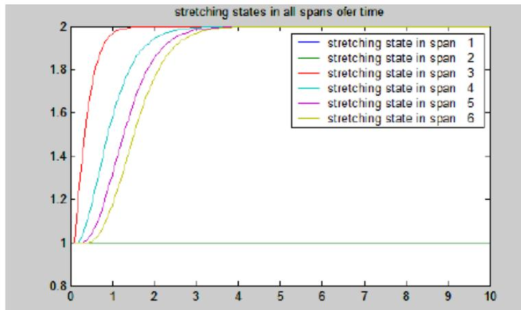
It can be seen, that starting at state 1 (no elongation): each span gets the stretched film later.
