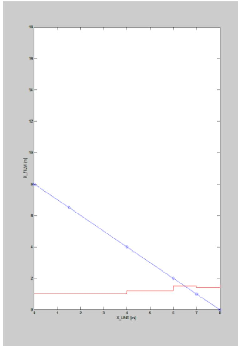
The blue line shows the  $x_{\text{film}}$  over  $x_{\text{line}}$ . In the first step this is a -45 degree line: no stretching of film at all. To make the starting point easy to understand, we have deliberately chosen the point, when the film length ( $x_{\text{film}} = 0$ ) has reached the end of our line ( $x_{\text{line}} = 8\text{m}$ ).
