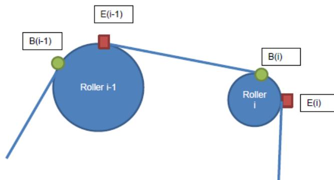
The film itself is transported by the rollers. The speed of the film between the rollers  $i-1$  and  $i$  is the surface speed  $f_i$  of roller  $i$ , that means the speed of the span is the surface speed of the next (downstream) roller. [Reference Brandenburg or other] The speed of film on the roller  $i$  is also the surface speed of the film on that roller.
