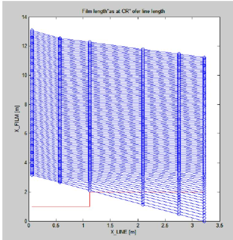
The stretching states before each roller (span):
